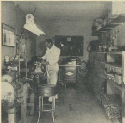
*Head and valve department, under Harold Daigh, has the job of making sure that all valves, seats, springs and combustion chambers for 335 engines are to top specs for high performance.*
