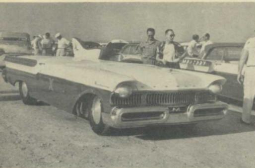
When ready to run at Daytona Beach, Florida, the "Mermaid" used Firestone 'Bonneville' tires and attracted much spectator attention. Best one-way speed was 159 mph with 154 mph average but later in the week, Art reported the tach reading nearly 180 mph when a radiator hose blew, spraying engine.
