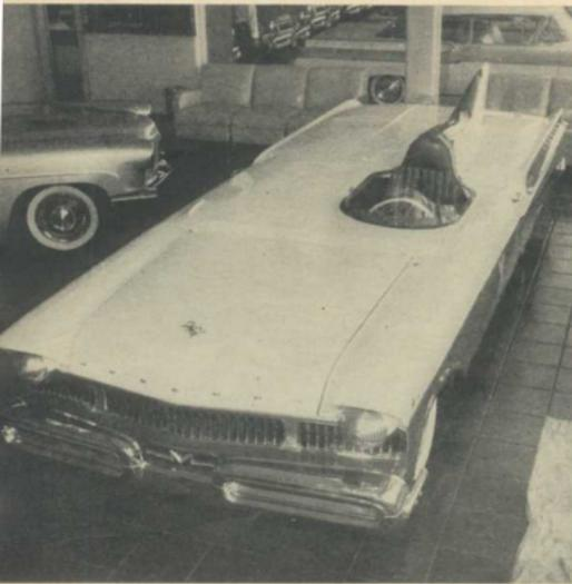
To get the near streamliner appearance of the "Mermaid," Bill Stroppe's crew cut the windshield glass and frame off a 1957 Mercury convertible, then had race car builder Eddie Kusma form an aluminum canopy with fin-tailed headrest for driver.
